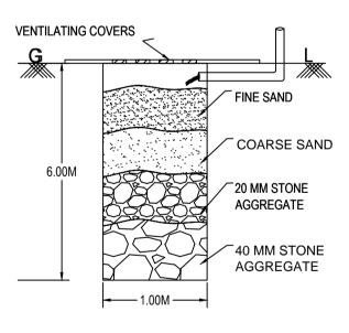
RAIN WATER HARVESTING STUCTURE DETAILS
